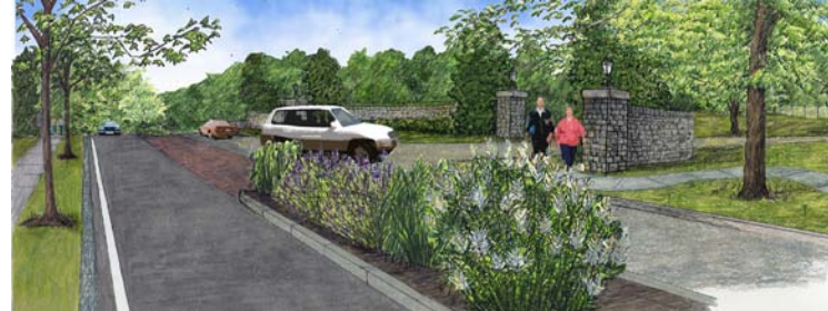
Option C6: splitter island for traffic calming with sidewalks and buffer area
