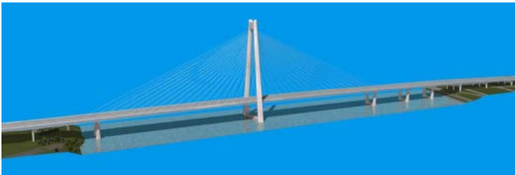
Alternative 1: Single Tower Cable-Stayed
